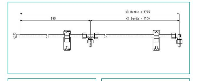
Acetylene Bundle manifolds are permanently installed high pressure lines with connection tubes, mounting consoles and connections for the bundle connecting hose. For use with connecting hose for acetylene order no. 910222.
